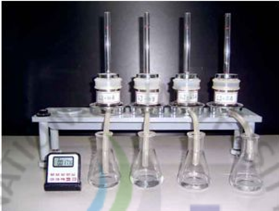
Fig. 6. Apparatus for measuring the hydraulic coefficient by falling head method.
