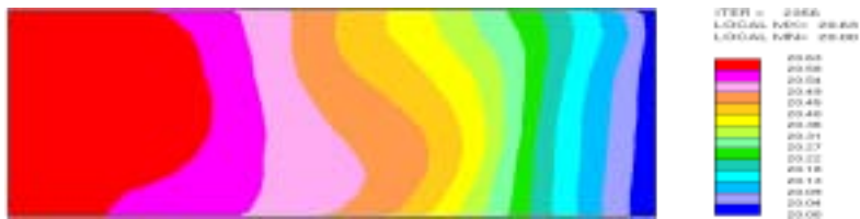
Fig. 45 Case 1 temperature contour of solidifying
