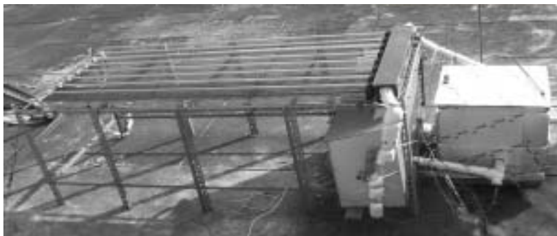
Fig. 18 Photograph of the installed single vacuum tube with a dual pipe flow passage(SEIDO 2)
