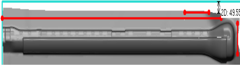
Fig. 92 Blank size & Metal flow(2st draw)
