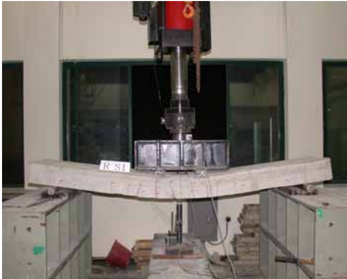
Fig 4.13 Shear compression failure(RS1)
