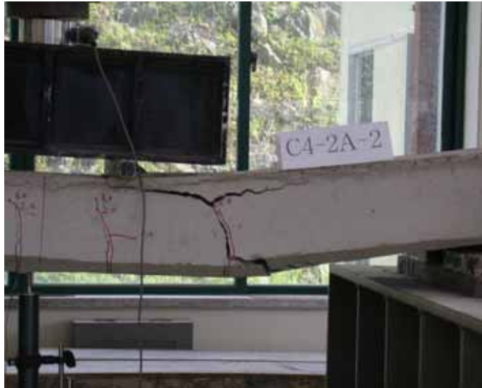
Fig 4.5 CFRP grid rupture failure
