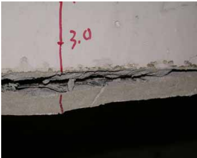
Fig 4.18 Interfacial debonding failure(C6A-2T-2)
