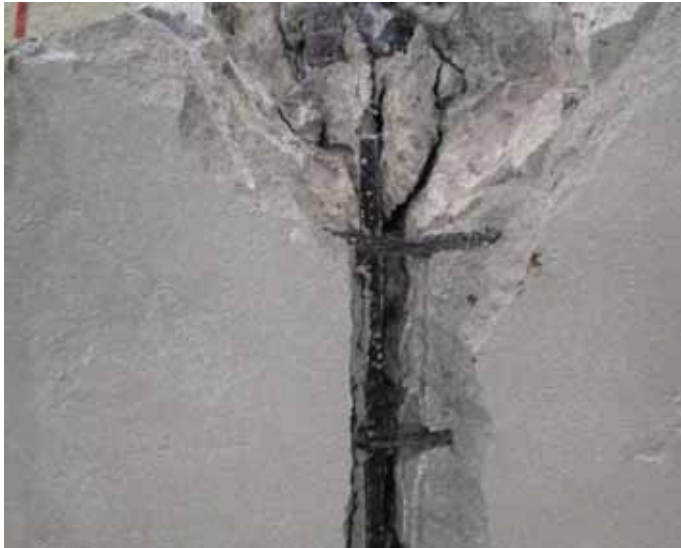
Fig 4.15 CFRP grid rupture(C4A-2T-1)
