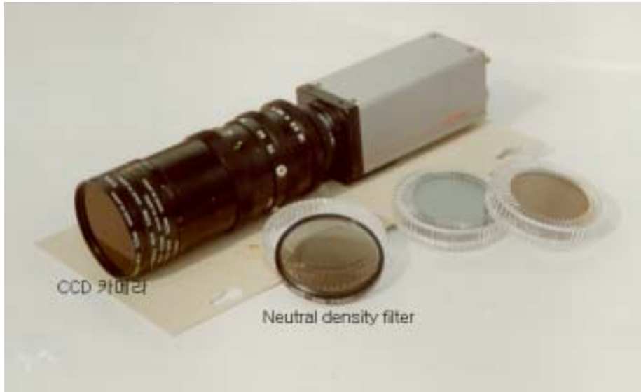
Fig. 3.4 CCD camera and neutral density filters
