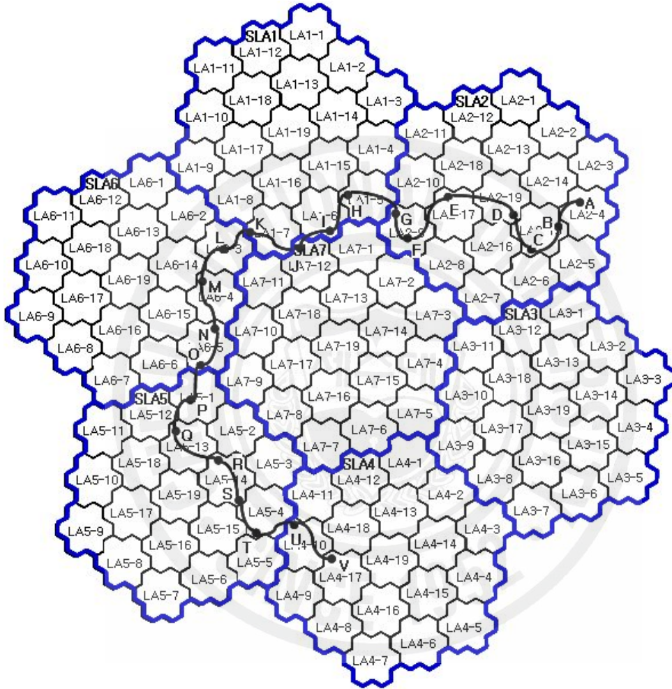
Figure 8. Moving Path of a mobile station in the SLA scheme
