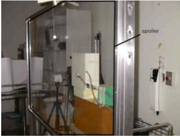
Fig. 22. Photograph of the spoiler setting.
