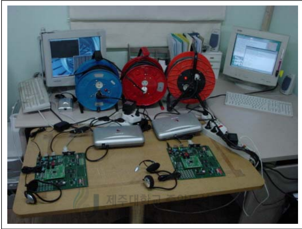
Fig. 18. Realization of VoIP using PLC
