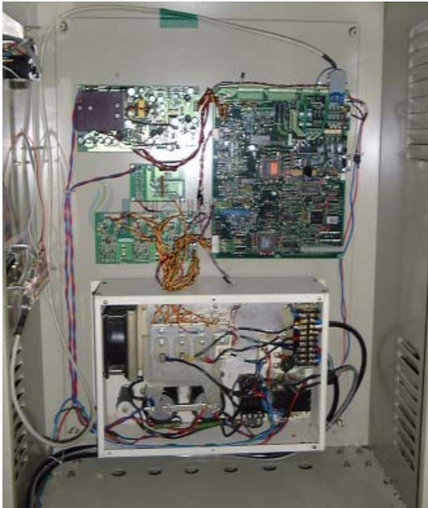
Fig. 9 Photograph of DSP and inverter system
