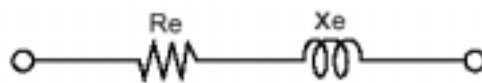
Fig. 5 Equivalent circuit of a piezoelectric ceramic resonator in the frequency band f_r \leq f \leq f_a
