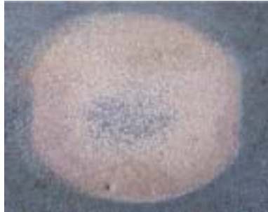
(b)500 hours corrosion
