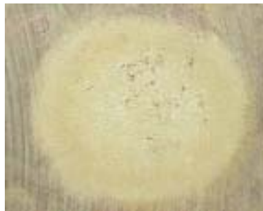
(c)1000 hours corrosion
