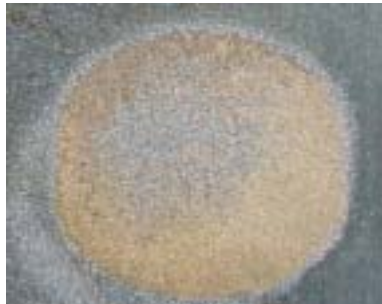
(c)1000 hours corrosion
