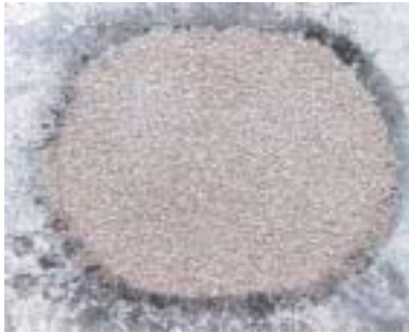
(c)1000 hours corrosion
