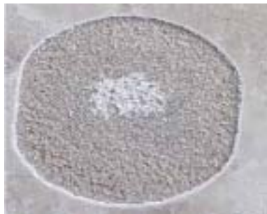
(c)1000 hours corrosion
