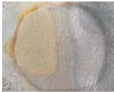
(b)500 hours corrosion
