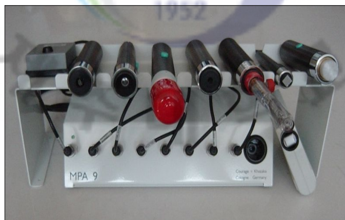
Figure 5. MPA9 system with various sensor probes.
