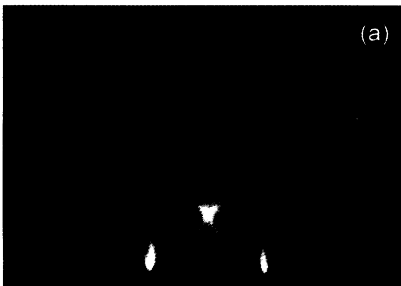
Fig. 4-1. (a) RHEED pattern taken from Si(111) surface held at room temperature after Co deposition 0.76 ML.
