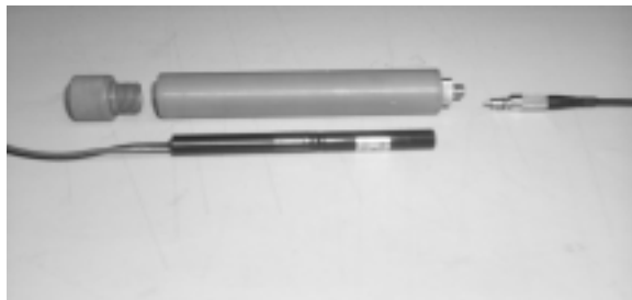
Fig. 26 PMT case used to fix transmitting fiber on the window of PMT.
