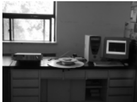
Fig. 15 Detecting system for optical fiber bending loss.
