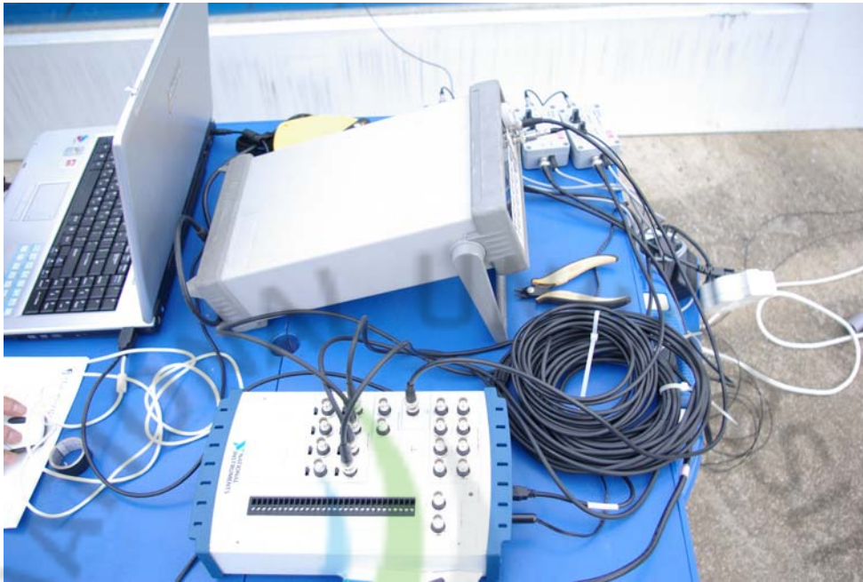
Fig. 22 SBL system installation for basin test
