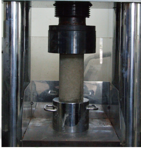
Fig. 3.3 Compressive strength test
