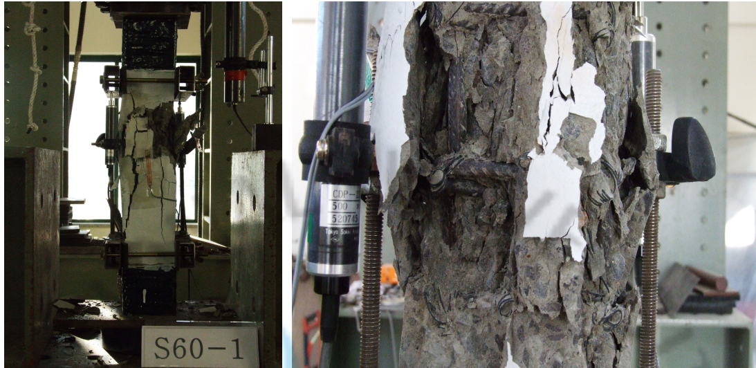
(a) Final failure and crack (b) Buckling of main reinforcement
