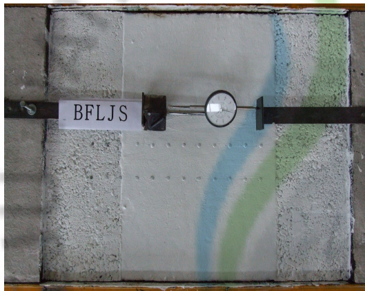
(a) Test set-up before experiment (b) Deformation pattern at surface
