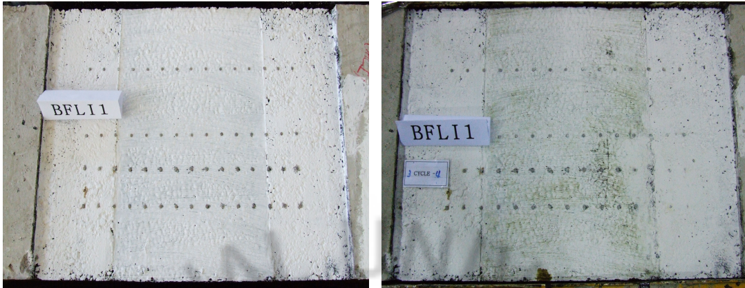
(a) Test set-up before experiment (b) Deformation patterns at surface
