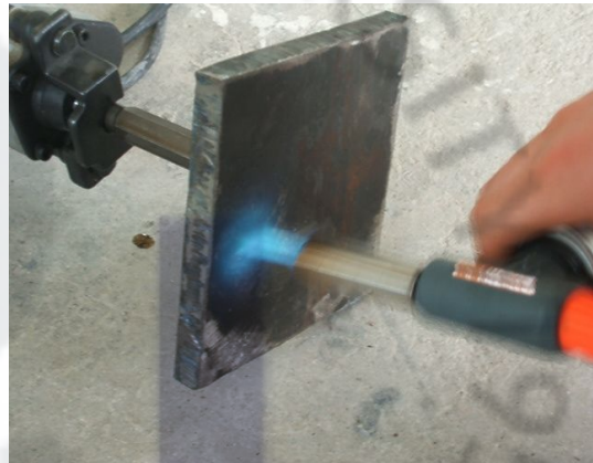
(f) Heating of compacting plate
