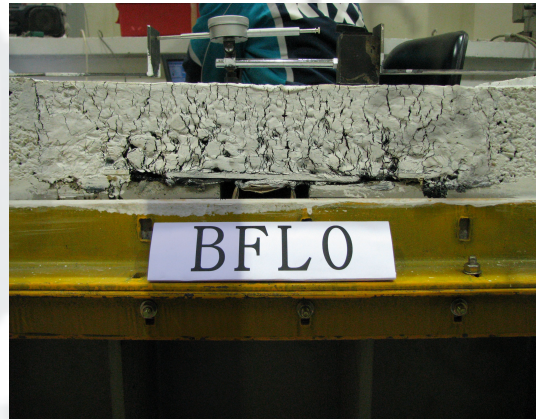
(c) Deformation pattern at cross sections
