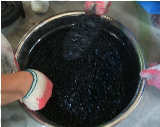
(e) Mixing of aggregate and asphalt
