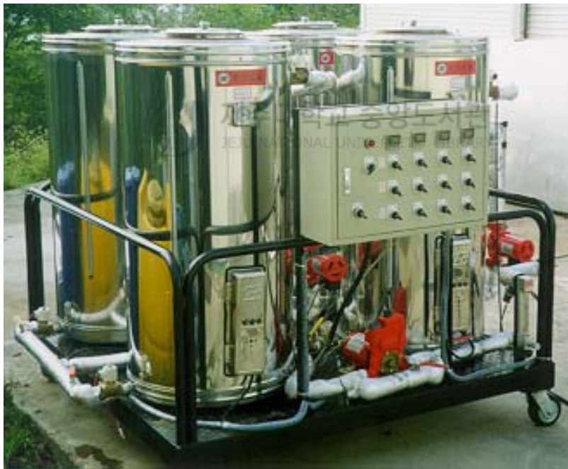
Fig. 5 Hot water supplier
