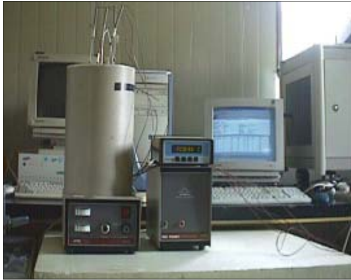
Fig. 1 Photograph of thermocouple calibration
