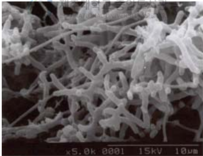
Fig. 3. SEM photographs of surface of activated carbon/polyurethane composite media (a) and microorganisms attached on composite media (b).
