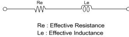
Fig. 8 An equivalent circuit of a piezoelectric ceramic resonator in the frequency band f_r \leq f \leq f_a
