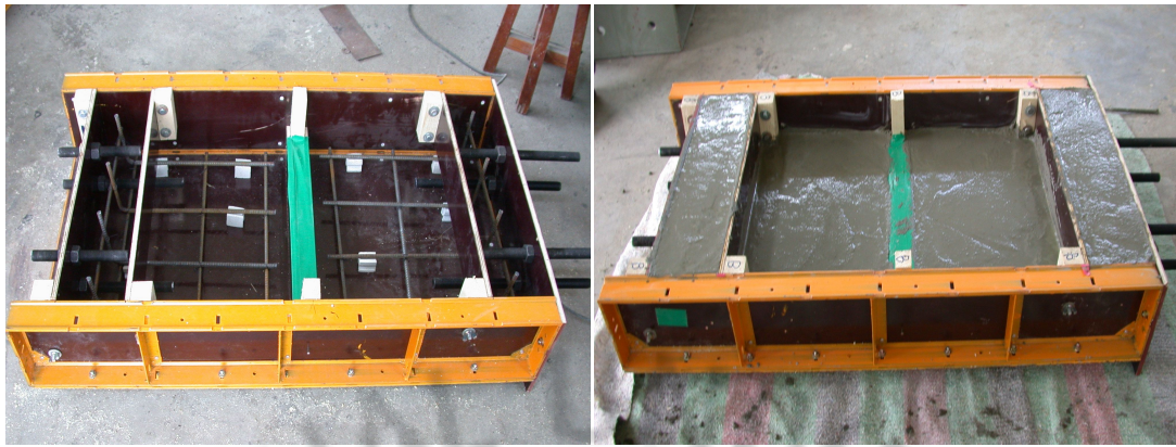
(a) Reinforcing bars in uroform
