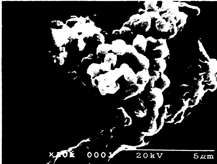
Fig. 15. SEM photograph of Hyphomicrobium spp. in biofilm reactor
