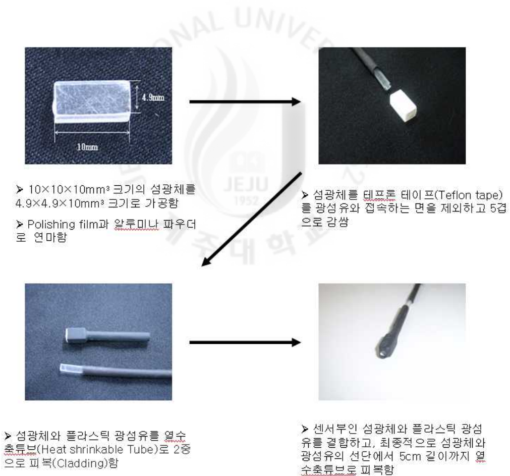
Fig. 9 Process of sensor manufacture
