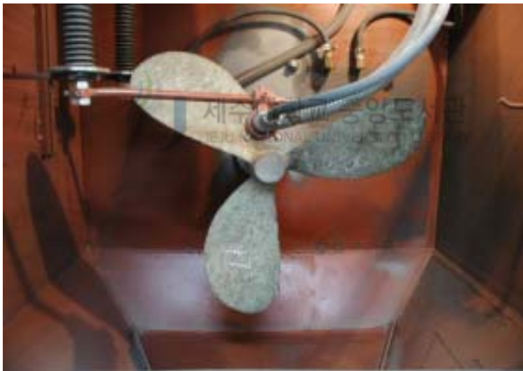
Fig. 64 An installed propeller in chamber of corrosion removing apparatus
