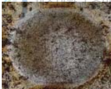
(C) 1000 hours corrosion
