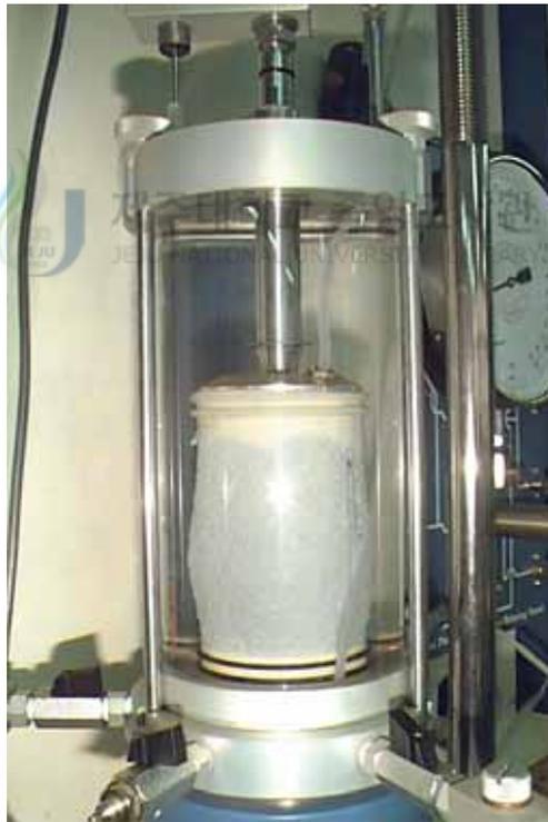
Fig 4.3 Central Bulging of Specimen during Triaxial Test.
