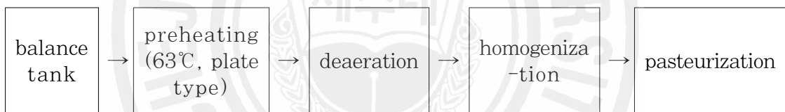
Fig. 7. Processing overview of sudachi juice pasteurization.
