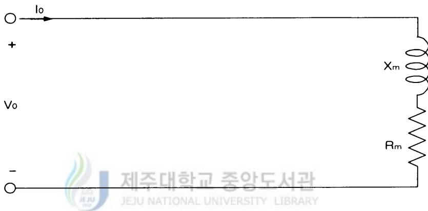
Fig. 2 Simplified no-load equivalent circuit
