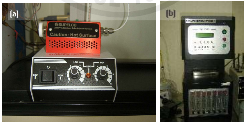
Fig. 13. ATIS (a) and Cleaning system for adsorption tube (b).
