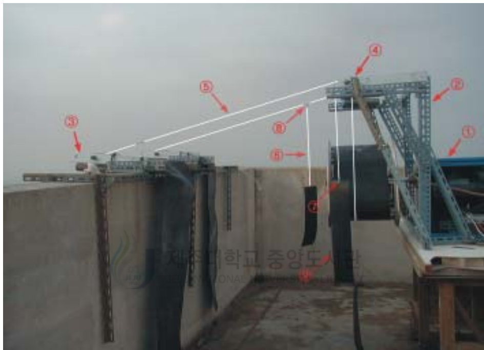
Fig. 3-9. Photograph of the rotary equipment for revolving a main line of the continuous hairtail hand line.
