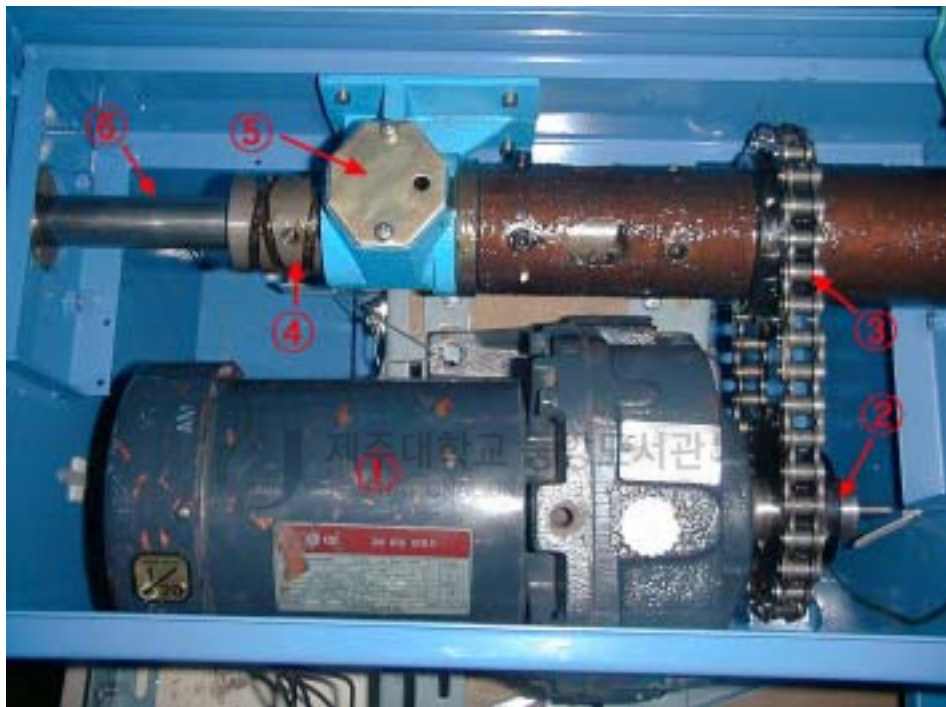
Fig. 3-16. Photograph of the rotary device renovated for the continuous hairtail hand line.
