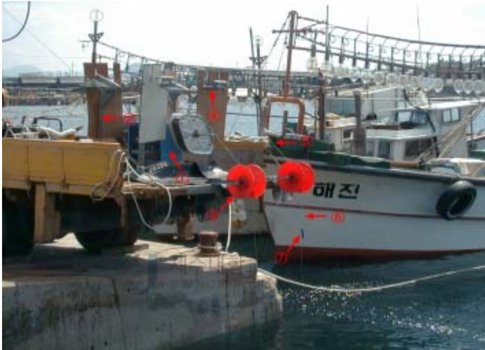
Fig. 3-13. Photograph of the rotary device for revolving a main line of the continuous hairtail and squid hand line.
