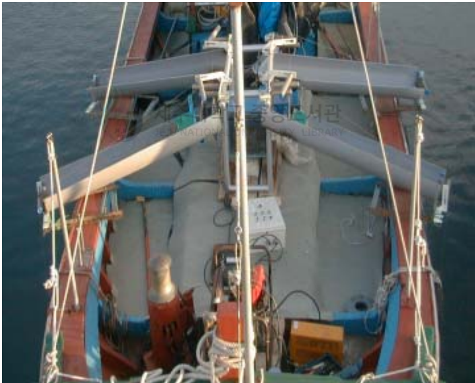
Fig. 15. The production of automatic hairtail hand line in the sea test.
