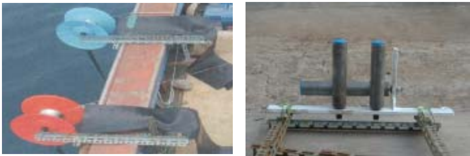
(a) (b) Fig. 6. The photograph of the side roller on the underwater model test and the sea test.
