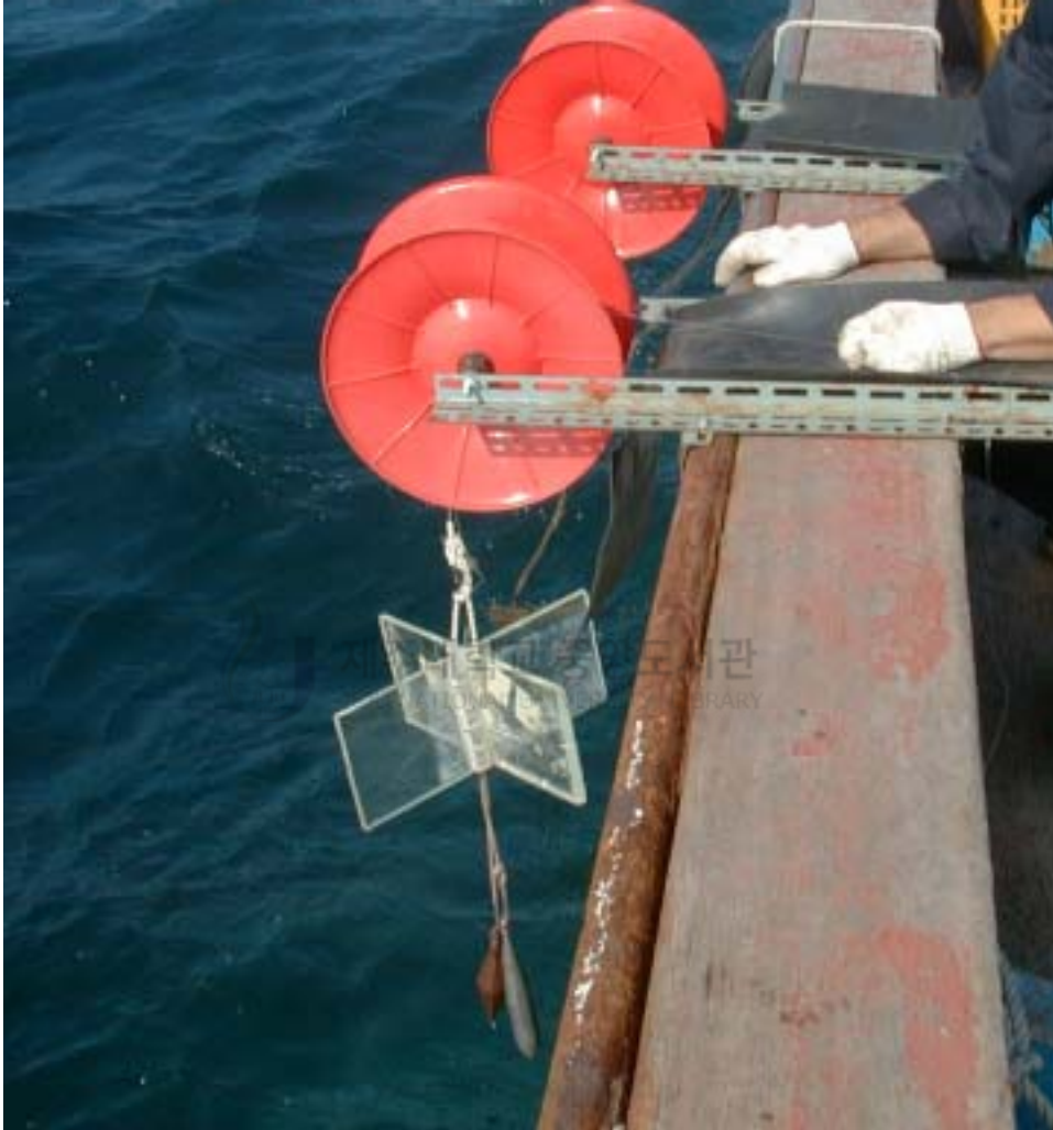
Fig. 12. The movement of resistance board in the sea test.
