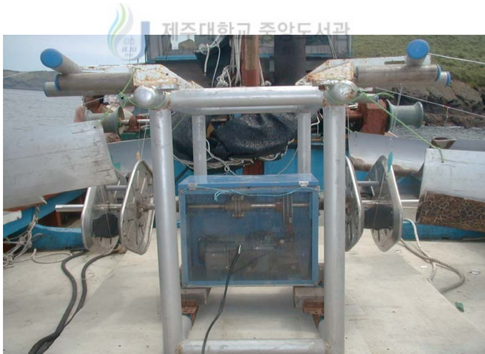
Fig. 6. The frame of continual squid hand line in the sea test.
