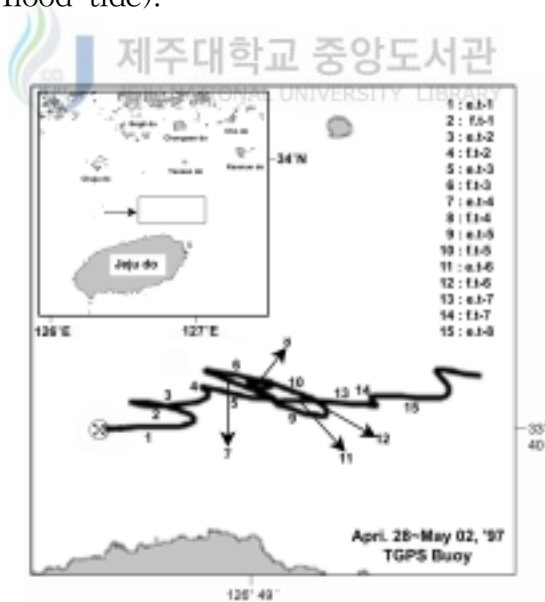
Fig. III-42. Drift track of TGPS Buoy in the northern sea area of Jeju do in Apr.28~May 02, 1997(e.t:ebb tide, f.t:flood tide).
