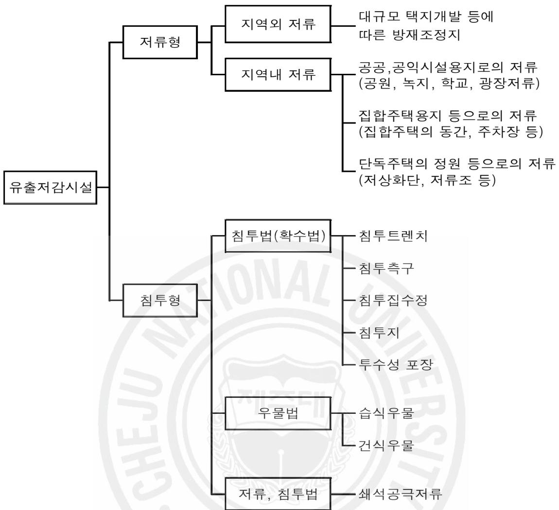
Fig 2.1 Types of the runoff reduction facilities
