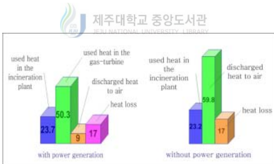
Fig. 2-3 Energy supply trend to each facility with or without operation of power generator at the Incineration Plant
