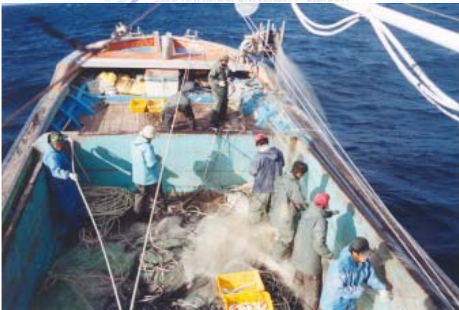
Fig. 22. The work scene to use quarter rope and Triple 'V' type net hauler
