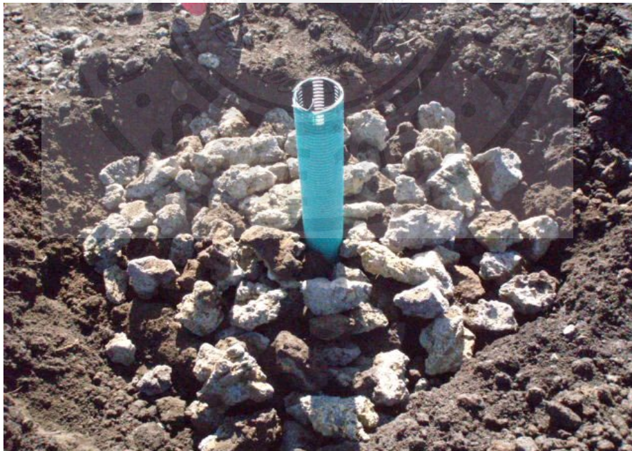
Fig. 4.3 The figure of Borehole Test with Constant Water Level
