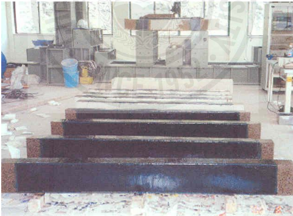
Fig. 3.11 CFRP sheet-bonded test beams
