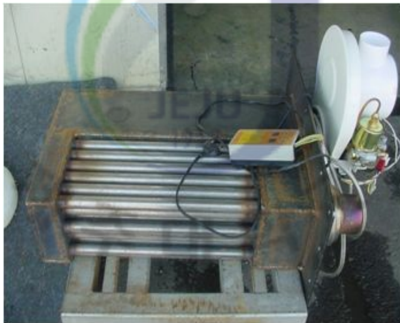
Fig. 2-5 Picture of heat exchange and burner
