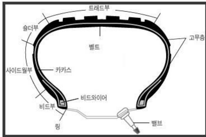
Fig. 2.5 General structure of the tire
