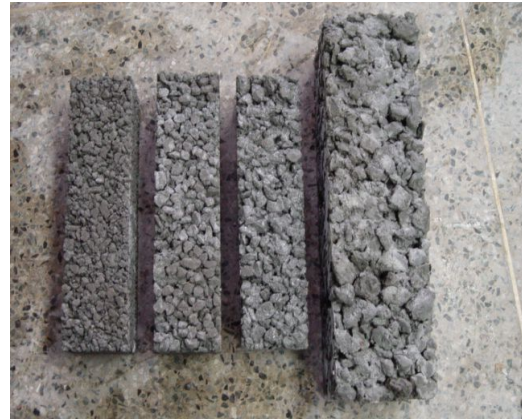
Fig. 4.5 The specimen for flexural strength with aggregate
