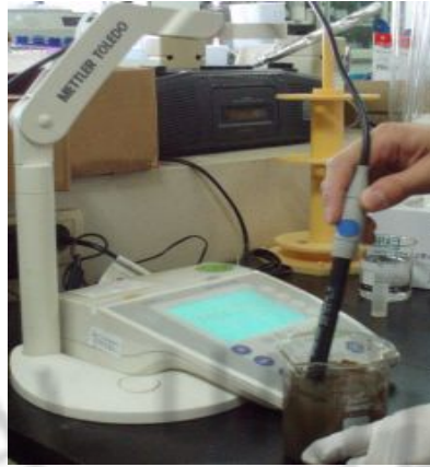
Fig 3.5 Photograph of pH test about Waste Concrete Powder
