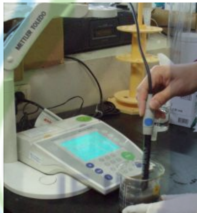
Fig 3.5 Photograph of pH test about Powdered Basalt
