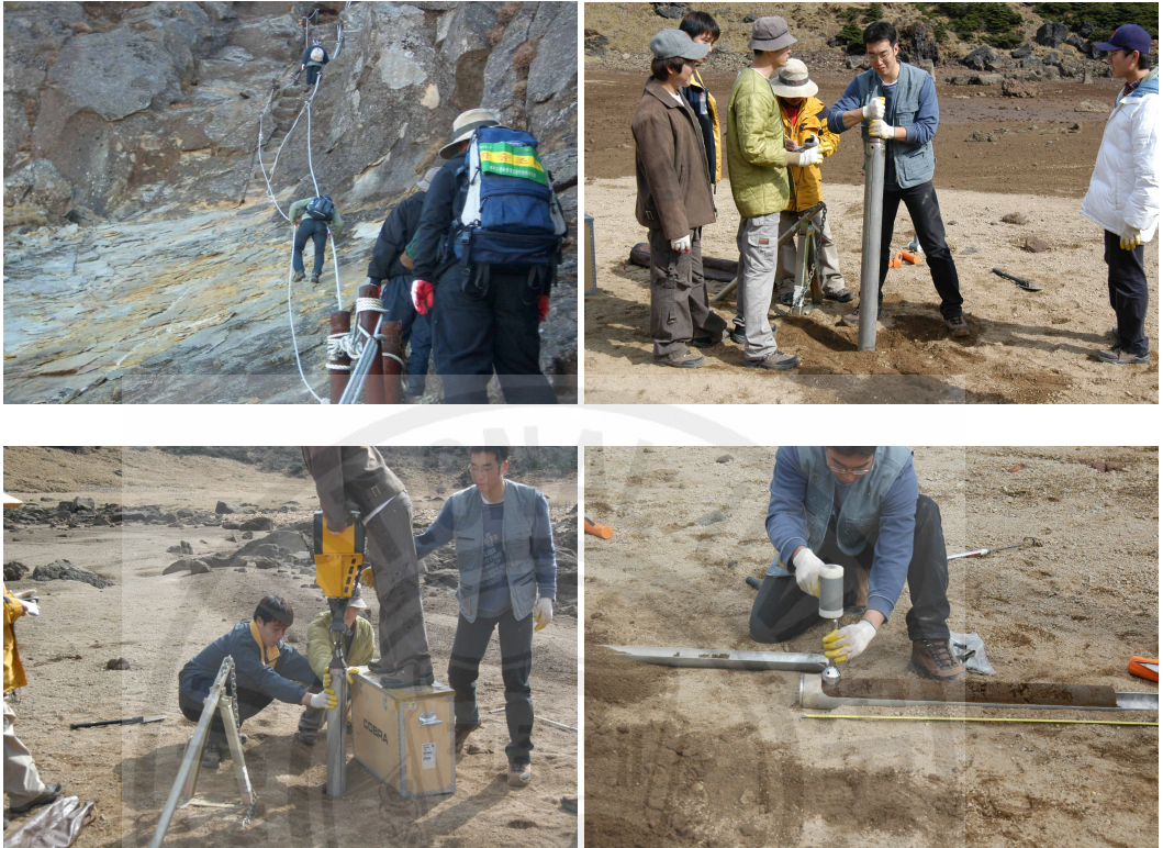
Fig. 2. Procedure of soil sampling with Cobra soil sampler in Baengnokdam crater lake.
