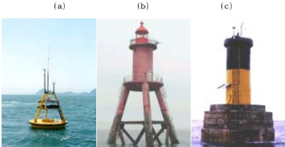
Fig. 2.1 The configuration of ocean data buoy in Dukjukdo(a), automatic ocean observation system at Seosudo(b), automatic ocean observation system at Gadaeam(c).
