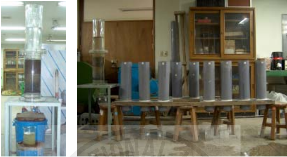
Fig. 6.1 Permeability Testing Mechanism for Indoor Model
