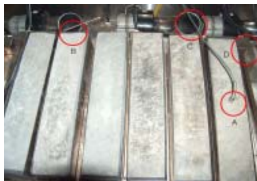
Fig. 4.54 The inside of freezing and thawing apparatus
