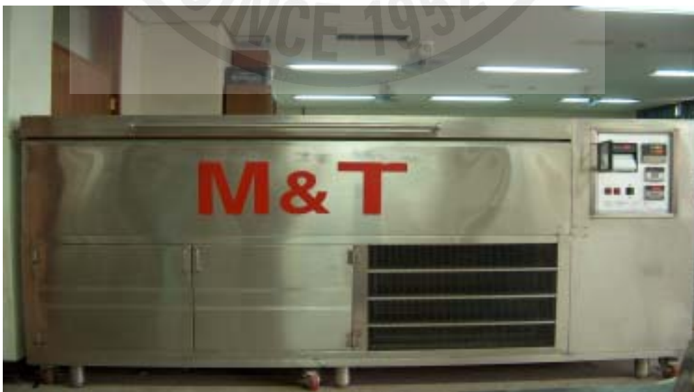
Fig. 4.52 Freezing and thawing apparatus
