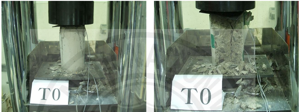
Fig 6.5 Failure mode (T0)
