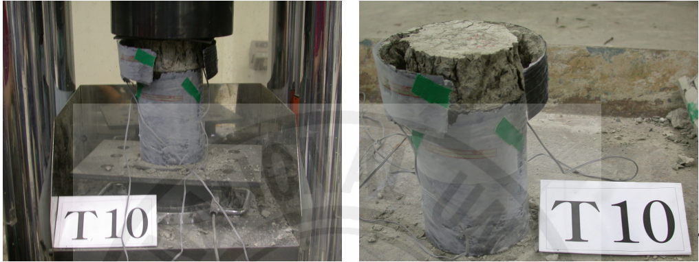
Fig 6.27 Failure mode (T10)
