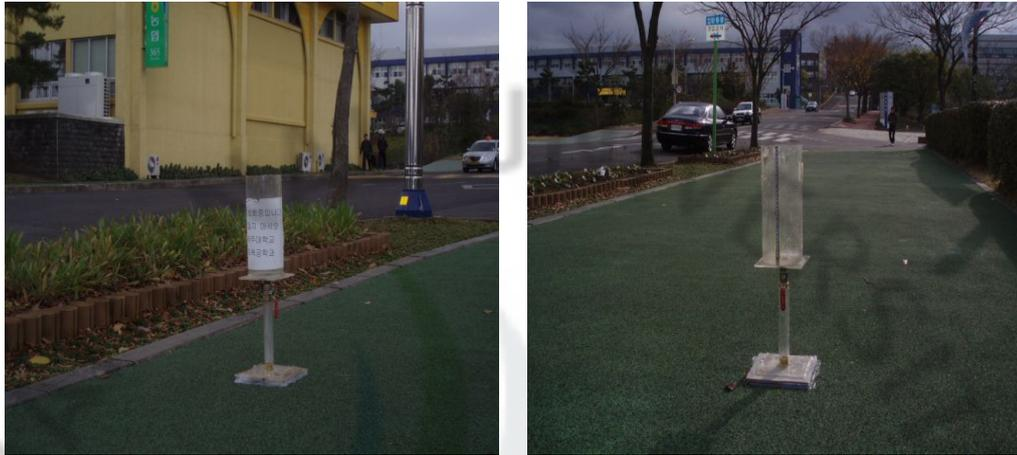
Fig. 4.36 Photograph of permeability test in field (porous elastic pavement)
