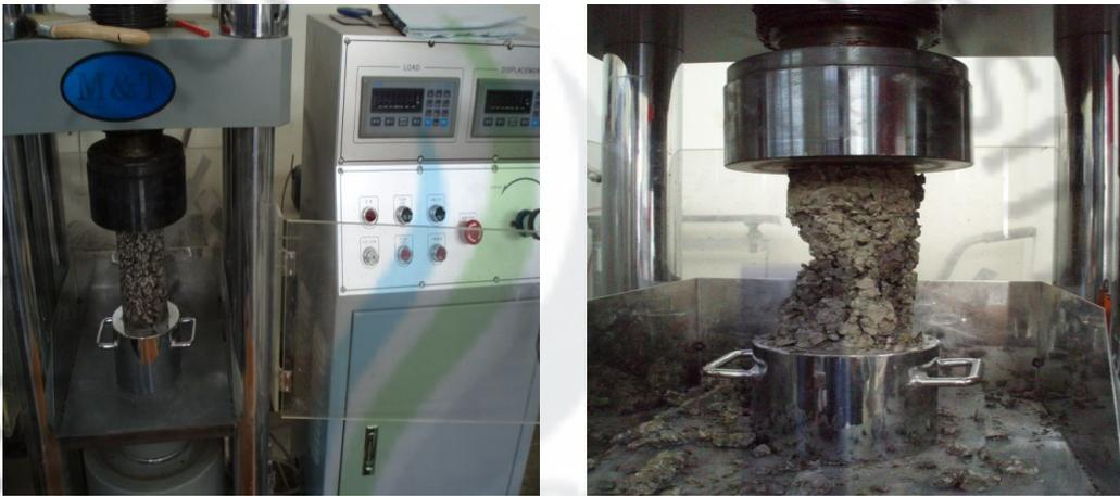
Fig. 4.1 Photograph of compression test
