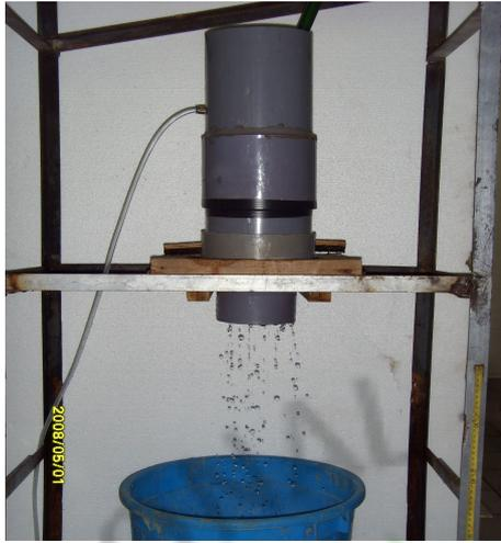
Fig. 4.11 Produced constant head permeability test apparatus
