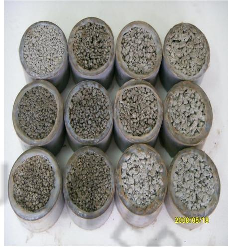
Fig 4.12 The test piece of permeability test
