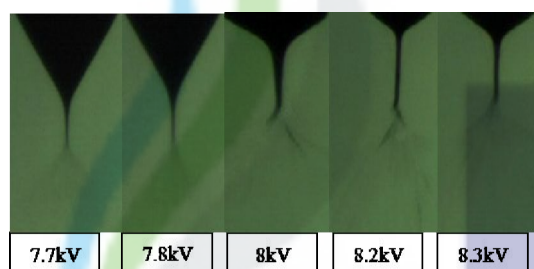
Fig.5.7 Different meniscus behavior of electro spray upon increasing voltage.
