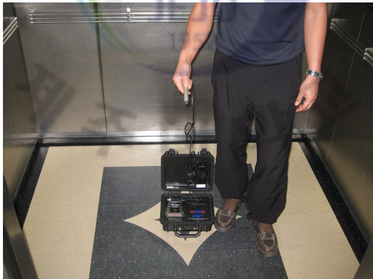
Fig. 5.23 Measurement of Vibration
