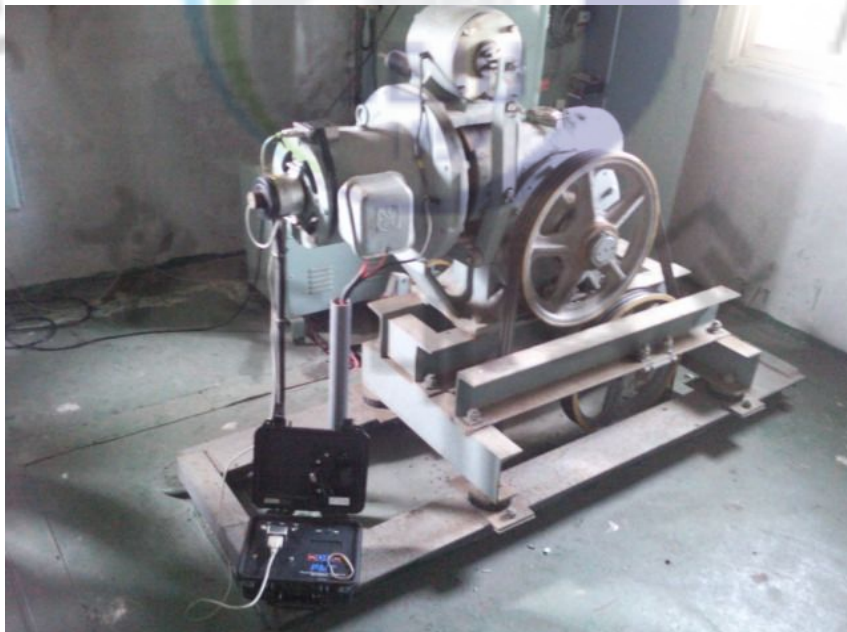
Fig. 5.7 Measurement of vibration
