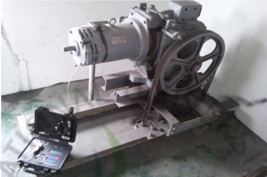
Fig. 5.3 Measurement of vibration
