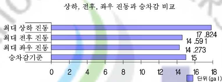
Fig. 6.3 Comparison Moving to-and-fro, left-right, up-down vibration & Comfort
