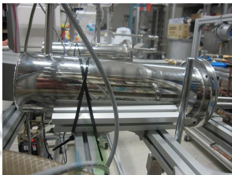
Fig. 28. Photograph of the condenser used in present experiment
