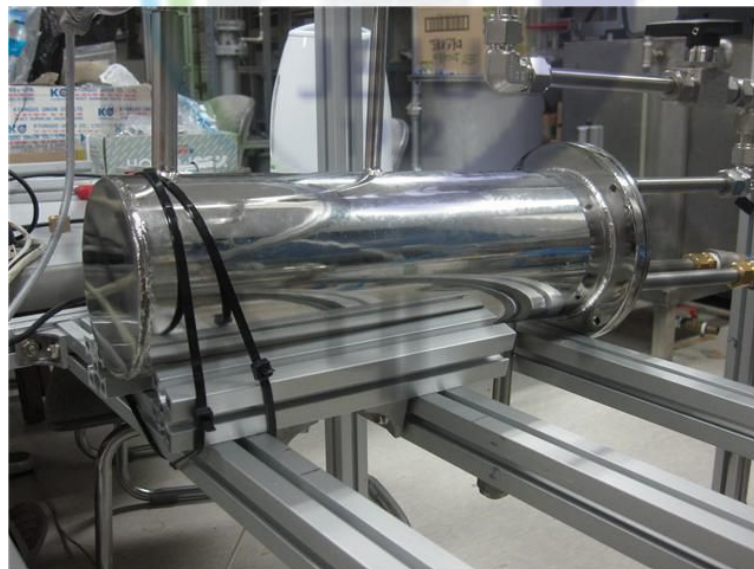
Fig. 24. Photograph of the evaporator used in present experiment
