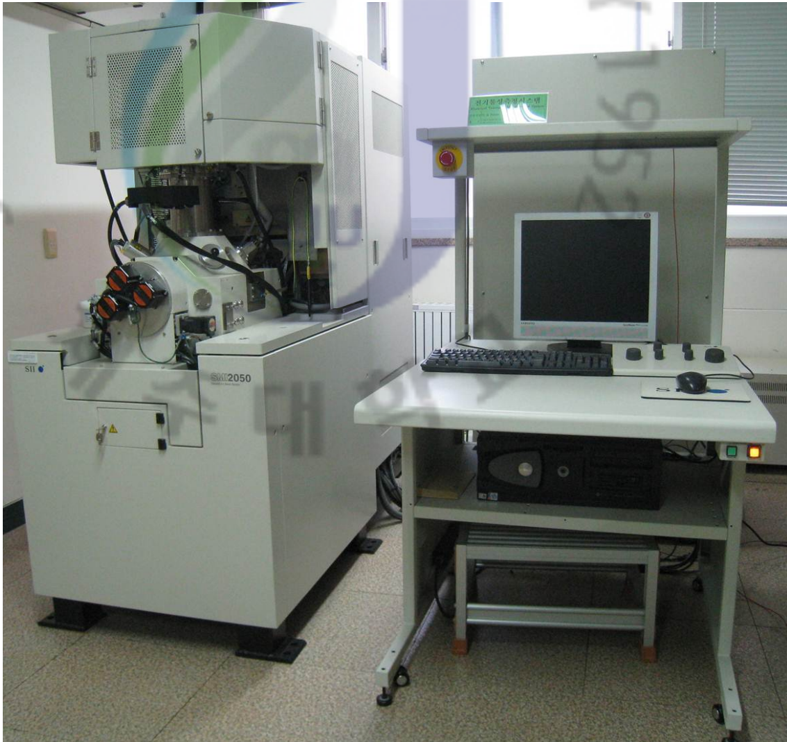
Fig. 3.2: A photograph of FIB machine (SII NanoTechnology SMI2050) in Research Instruments Center (RIC).
